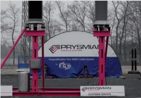
400 kV prequalification test, external laboratory.
